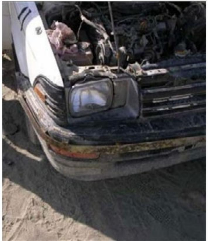
This suicide vehicle is equipped with a pressure activated bumper. The driver activates a switch inside the passenger compartment just before engaging the target.
